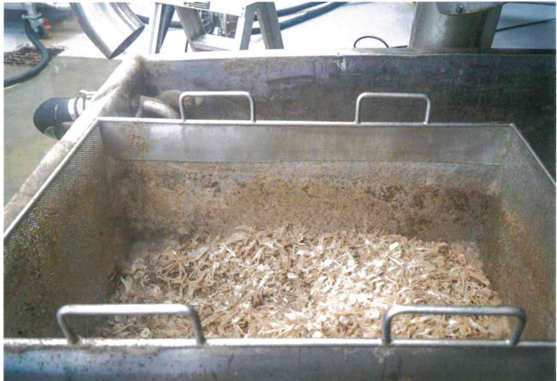
The dry extract once the fine mesh screen has done its job of separating solids from liquid.
